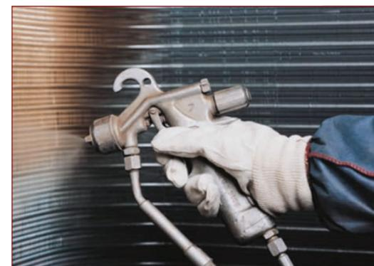
*Spray-on application of coating on new coil.*
