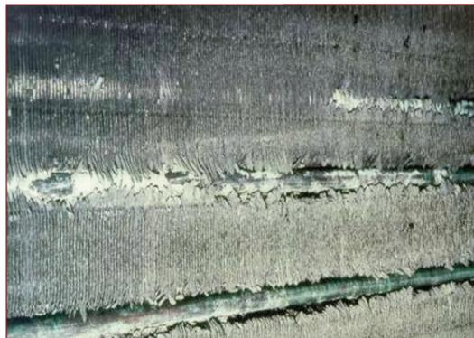
*Galvanic corrosion in existing coil.*
