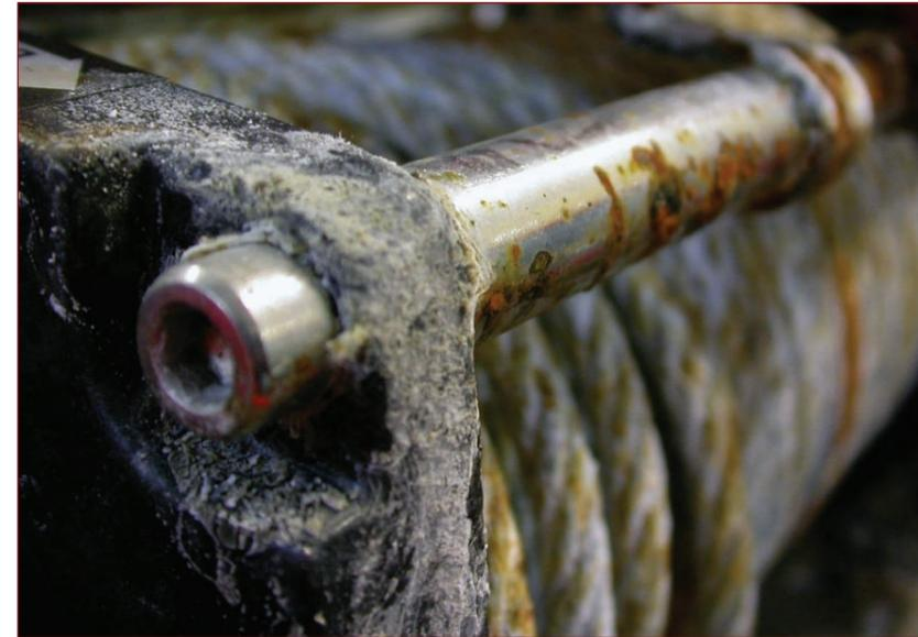
Corrosion damage on stainless steel, painted steel and galvanized steel surfaces after exposure to 500 hours of salt fog.
