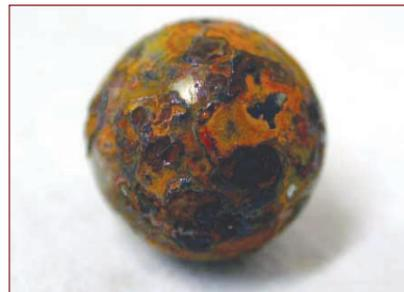
Corrosion of untreated steel ball. Salt fog exposure 240 hours.
