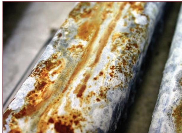
Surface corrosion and zinc oxidation on galvanised steel after exposure to 1000 hours of salt fog.
