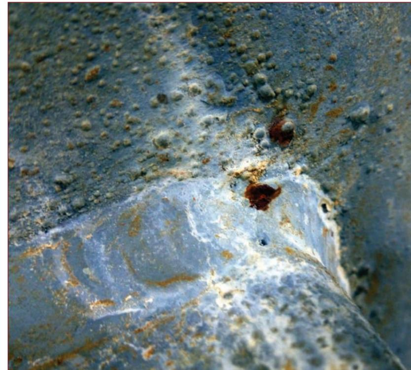
Corrosion failure on steel component coated with inorganic zinc. Total salt fog exposure 240 hrs.
