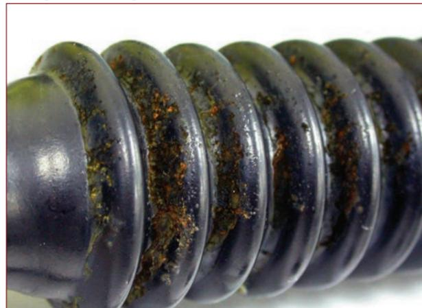
Condition of test panel after exposure to salt fog for 1000 hours. Steel coated with zinc. Note edge preparation.
