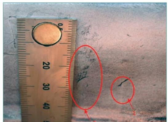
Image 1d: Corresponding test area after paint removal.
