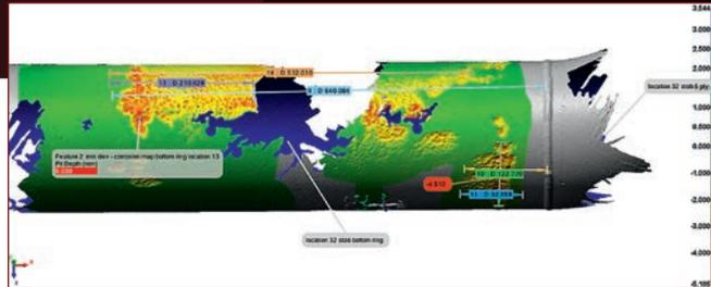
Figure 4. Post processing of the scan data produces deepest pit depths in full colour and 3D.
