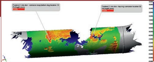
Figure 3. Using wireless technology the scan data can be closely monitored by the technician in real time.
