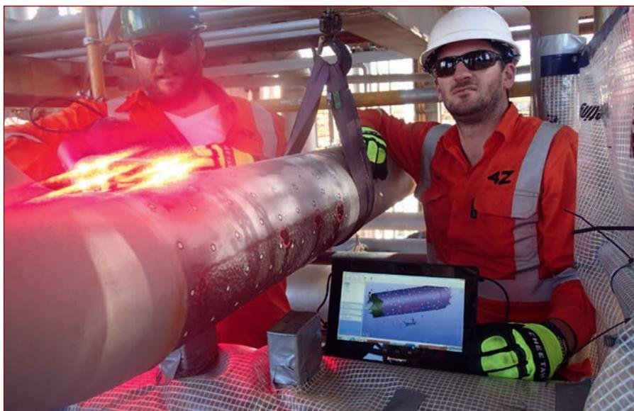
Figure 5. Further post processing can go to a level 2 assessment, detailing the geometry of the corrosion feature.
