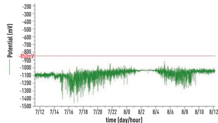
Figure 2: DC Stray Currents Recorded Over a 24 Hour Period.
