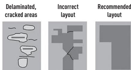
Figure 1: Concrete Repair Geometry.
