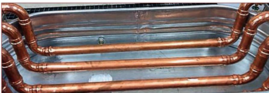
Figure 2: Test trough with bare copper pipes.
