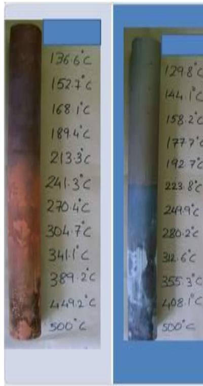
**Figure 4** – Comparison of Bis A Epoxies after dry heat testing
