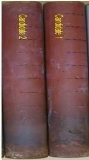
**Figure 8** - Comparison of Bis A Epoxies after CUI testing
