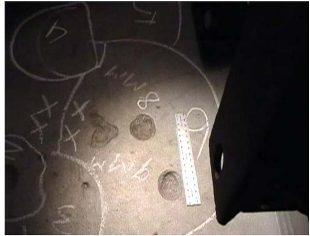
**Photo 4- Bilge Plating-pitting corrosion**
